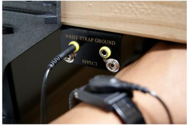
potentiometers, and aluminum parts, there would only be safety issues related to electricity. To be safe, my brother and I have built an electrical engineering lab in the loft. Attached to this lab is a wrist strap connected to the ground to prevent static discharge to electronics.
