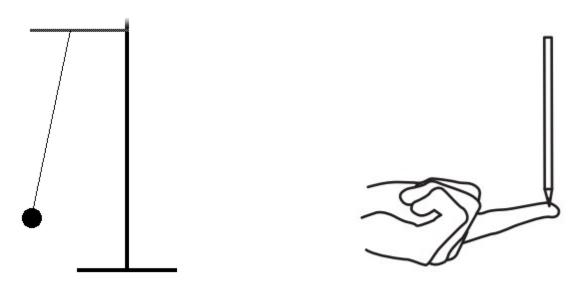
On the other hand, an inverted pendulum is a weight balanced on top of a light rod; it's the same system, turned upside-down. An inverted pendulum is the embodiment of an unstable, not robust system. When given even the smallest inputs, or disturbances, the inverted pendulum isn't able to return to its equilibrium state. It's the definition of a balancing act.
